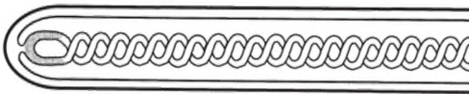
Fig 10: Fabricated Thermocouple Insulated, Twisted Pair Thermocouple inside Stainless Steel Sheath. Measuring junction earthed in this example.
