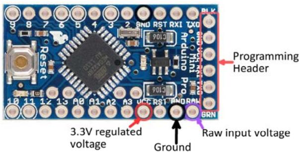
There are three different power-related pins: GND, VCC, and RAW. GND, obviously, is the common/ground/0V reference. RAW is the input voltage that runs into the regulator. The voltage at this input can be anywhere from 3.4 to 12V. The voltage at VCC is supplied directly to the Pro Mini, so any voltage applied to that pin should already be regulated to 3.3V.
