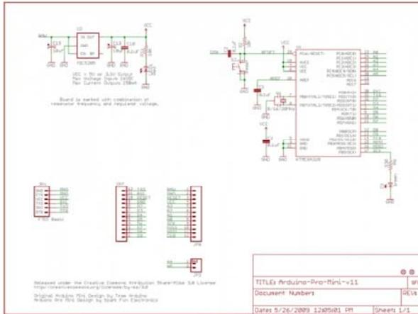
The Pro Mini's pins surround three of the four sides. The pins on the short side are used for programming, they match up to the FTDI Basic Breakout. The pins on the other two sides are an assortment of power and GPIO pins (just like the standard Arduino).
