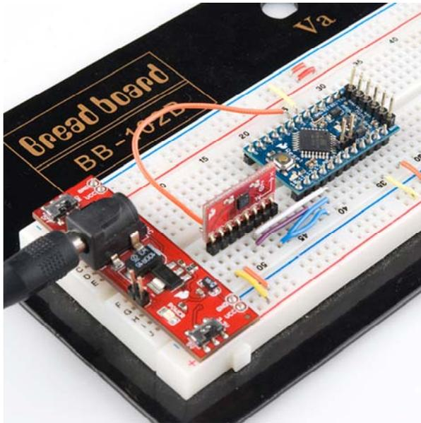
*This Pro Mini had male headers soldered into all pins, so it could slot directly into a breadboard. Notice the programming header pins are soldered "upside-down", to keep them accessible.*
